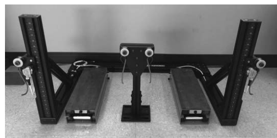
Figure 3: Laser measurement system for toe and slop in manual wheelchairs
